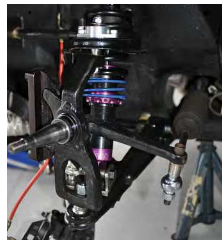
TOP: Lap Analysis via V-Box to finesse both chassis and driver. MID RIGHT: Alfa 6 Upright with Quantum coil-over, CSR upper ball joint and reversed ball joint lower arm.
