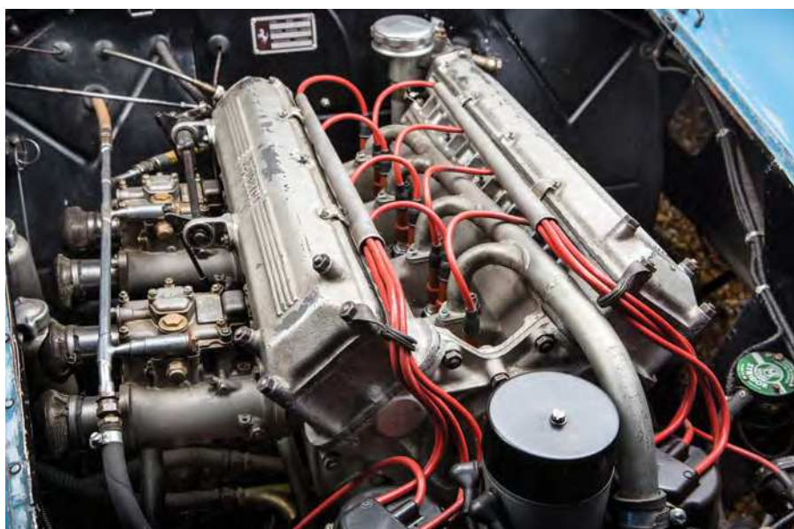
Scaglietti-bodied Series 2 Tipo 500 Mondial. Now with coil ignition rather than magnetos, the S2's Tipo 111 four had a much wider overhead valve 'vee'
